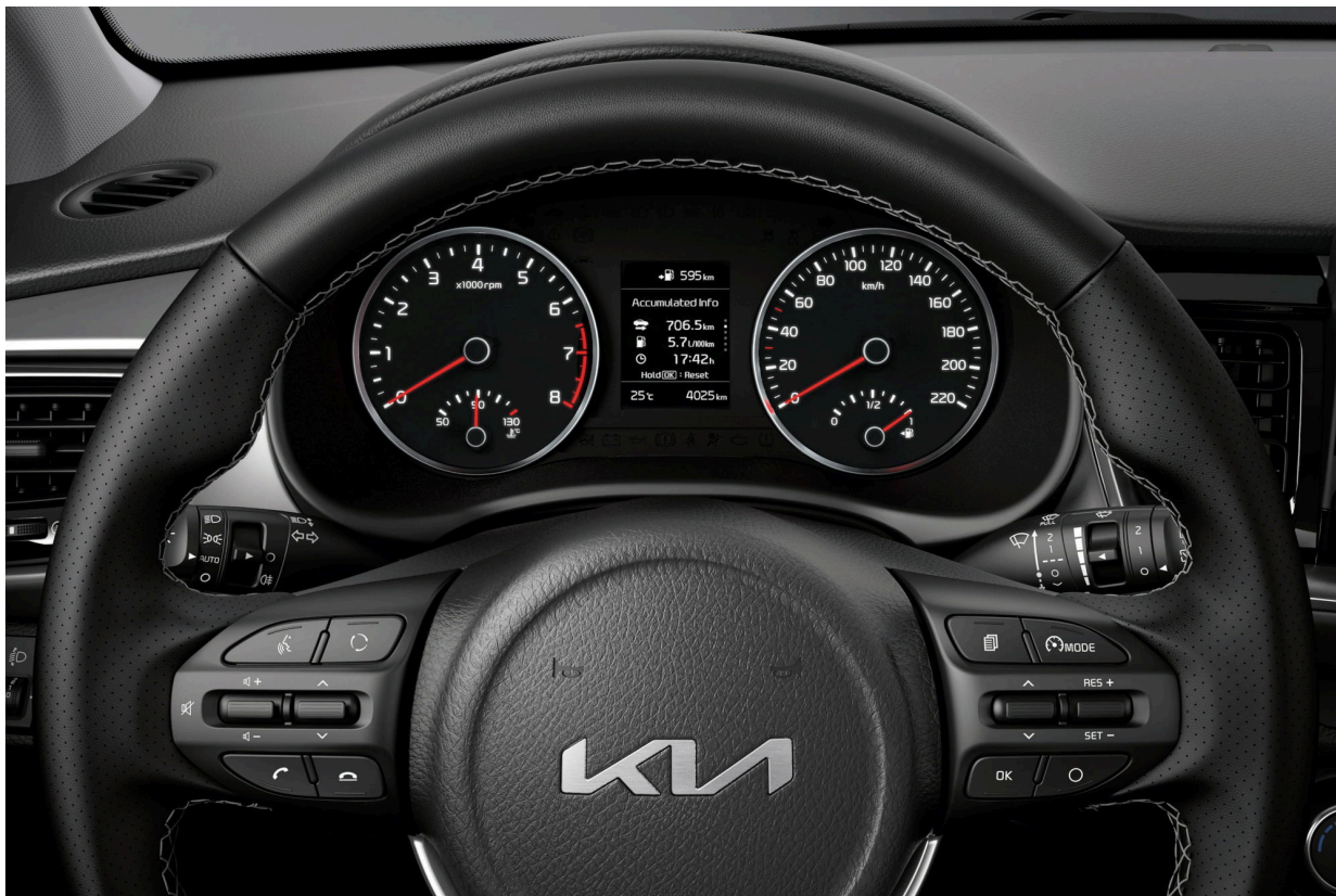
4.2-inch colour supervision cluster. Between the speedometer and tachometer, the screen displays vehicle status, audio information and gives you access to vehicle setting menus.
