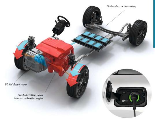
WITH HYBRID TECHNOLOGY, YOU BENEFIT FROM A LATEST-GENERATION INTERNAL COMBUSTION ENGINE, FUEL ECONOMY, A POWERFUL ELECTRIC MOTOR AND EFFICIENT ENERGY MANAGEMENT
