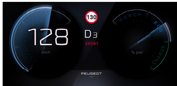
The digital speedometer (image shown is for New 208 Electric variants, displaying numbers in metric system.)
