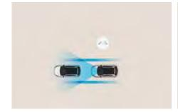
Lane Follow Assist (LFA): Smart sensors and the forward-facing camera detect when the car drifts from the centre of the lane, applying steering torque to hold road positioning for safety. The car also estimates the trajectory of the vehicle ahead and adjusts its position accordingly. Standard on Premium models.
