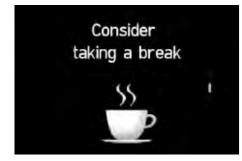
Driver Attention Warning (DAW): When a pattern of Front Collision Avoidance (FCA): The front view fatigue or distraction is identified, the system gets your attention with an alert and pop-up message suggesting a break.
