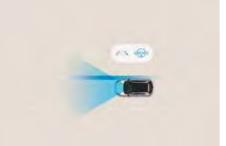
Lane Keep Assist (LKA): The Lane Keep Assist (LKA) uses the front multi-function camera to monitor the lines of the road. In case of an unintended lane departure, it warns you and can apply counter steering torque to guide the car back to the lane.
