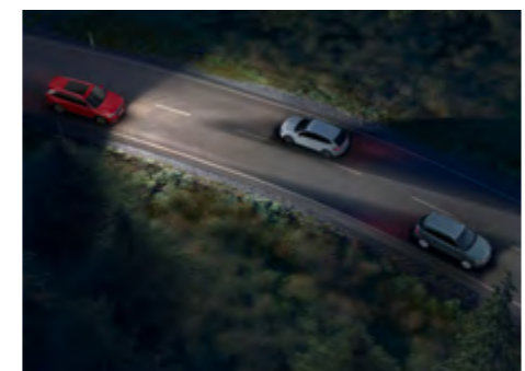
Full LED Matrix headlights with AFS (adaptive front light system), cornering function and AWL (all weather lighting system)
