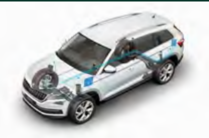
Dynamic chassis control Once selected, the vehicle will continuously evaluate the driving situation, adapting the damping and steering characteristics.
